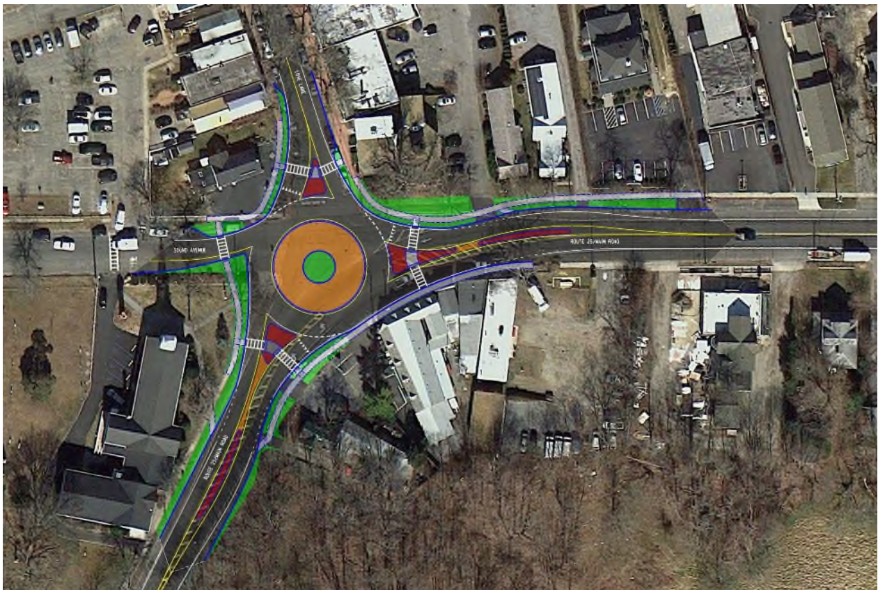
Figure 7: Alternative 3 – Roundabout Design by NYSDOT
